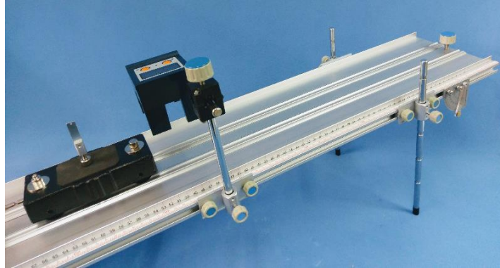
Figure 4-4 Schematic diagram of inclined plane movement device
