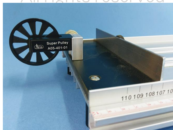
Figure 4-2 Fixed pulley device
