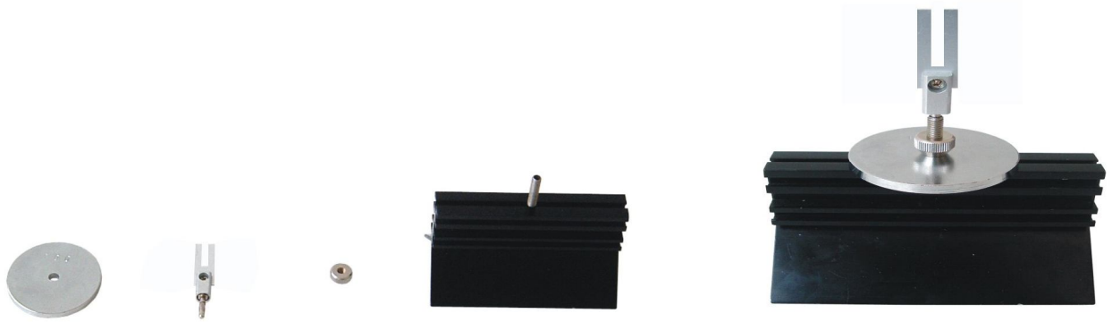
Figure 4-5 How to change the mass of the cart
