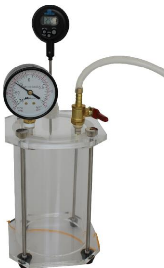
Figure 3-6 Vacuum pressurized cabin
