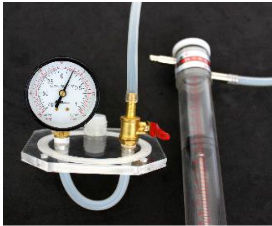
Figure 3-1 Pressure increasing device
