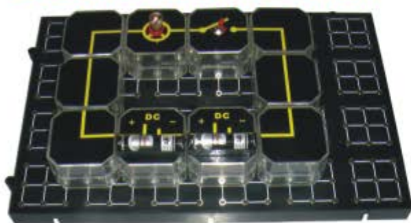
Experiment A : Open circuit and broken circuit
