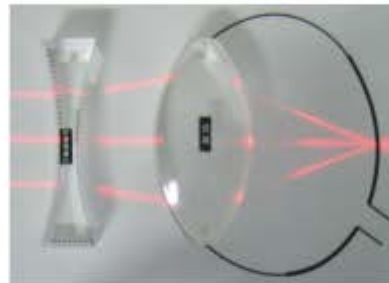
(Myopia: Cause and correction) Use concave lenses to focus light source on the retina.
