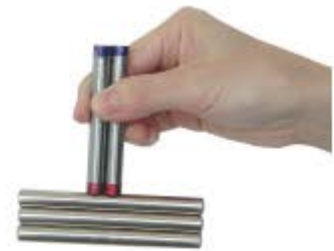
(Parallel repulsion) Magnetic force of the combination of same pole is greater than one magnet.
