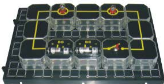
(Bulbs in series connection experiment)
