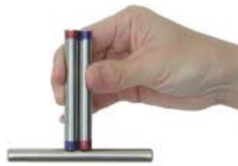
(Parallel attraction) Magnetic force of the combination of different poles is less than one magnet.
