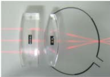
(Hyperopia correction) Use convex lenses to gather light source on the retina.
